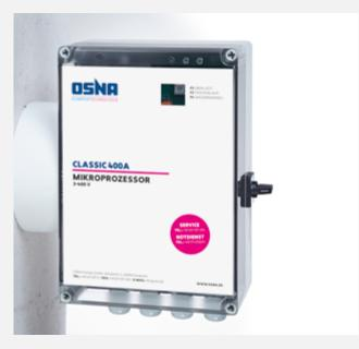
Electronic controller type Classic 400A, control and protection of direct starting single pumps up to 11 A at 400 V. The cointrol box is equipped with a digital display to communicate its operating condition.
